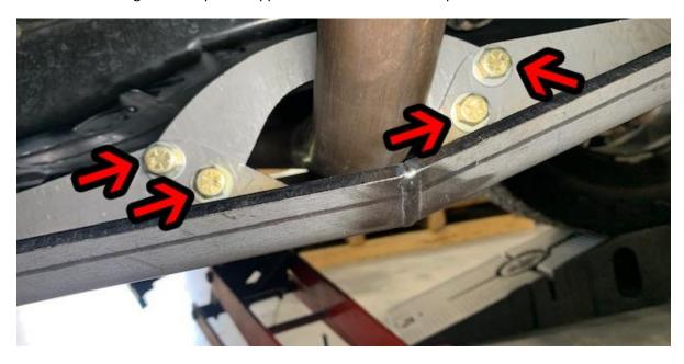
**Step 8:**Install the oil change door with its supplied hardware as shown below.
