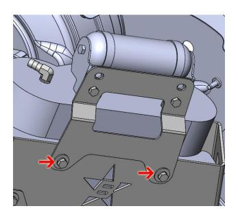
**Step 10:**Setup the control panel as shown below do not overtighten the ARB filters.
