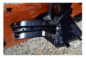
With the third brake light out of the way we now had to move to the inside of the tailgate and remove the vent inside the tailgate. This vent was a very tight fit and the left side has to be gently pulled out first in order for it to be removed.
