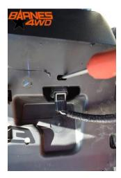
Now that we had the stock bracket removed 2 small threaded inserts had to be removed that 2 of the screws threaded into. We took a pair of needle nose pliers on the inside of the body and squeezed the two tabs on either side of the insert to remove it from the hole that it was installed in.
