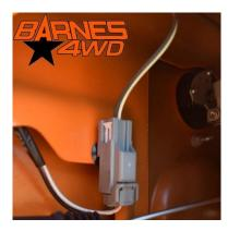
This plug had to be disconnected so we could remove the wiring harness for the third brake light as it will no longer be needed.
