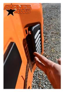
Here is the vent removed showing the clips that hold it in place
