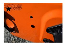
The factory tire carrier now had to come off, we used a 13 mm socket to remove the 8 bolts holding it on.
