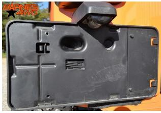
After these 4 bolts were removed we were able to access the plug for the factory license plate light. A small flat head screwdriver was used through a hole in the back of the bracket to release the clip holding the two halves of the plug together.
