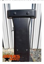
With the 4 screws removed we were now able to access the electrical plug on the backside of the third brake light, there is a small release that has to be squeezed and the plug will pull right out.
