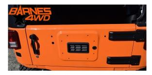
With the tire carrier out of the way the vent in tailgate needed to be removed, there were several tabs on the back that hold it in.
