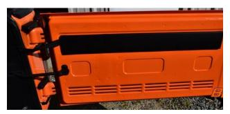
The backside of the panel showing the clips that have to be popped out of the tailgate.
