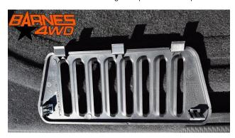
Removing the vent gained us access to the plug inside the tailgate for the third brake light wiring harness.
