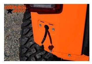
Here is what the clips look like after removal, you can see the small tabs that have to be squeezed to facilitate removal.
