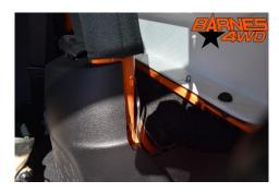
We were now down to the last panel, 2 bolts had to be removed and one nut had to be loosened. Two bolts go through the footman loops in the floor and we used a T30 Torx to remove them, the one nut is near the roll bar tube behind the interior panel a 10mm open end wrench was used to loosen it. After all of the fasteners were removed the panel still has two spring loaded clips on the backside, we pulled and popped the clips loose from there retainers and were then able to remove the panel.
