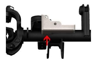
Step 11: Now that you have the Front Trackbar Bracket Welded into Place. Bolt your trackbar into place.
