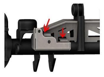
Step 6: Tack Weld the trackbar bracket into place.
