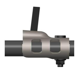
Orientation of stabilizer end will change. See picture below. Tighten the stabilizer bracket into place.
