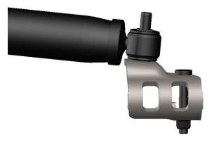
The Steering Stabilizer will mount to the outside of the trackbar bracket.
