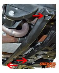
3. Using the same 18mm socket we removed the 2 bolts that secure the fuel tank skid to the cross member.
