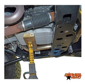
6. Using the 18mm wrench and the 18mm socket we removed the nuts on either end of the cross member (4 total).
