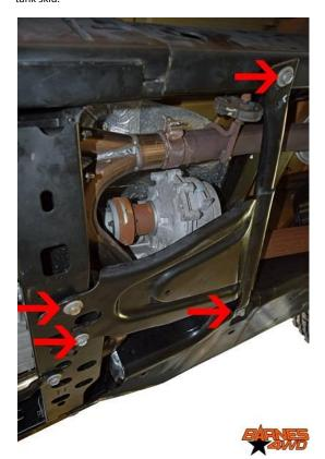
2. Using the 18mm socket again we removed the transmission pan skid. There was one bolt in either frame rail and one in the crossmember.
