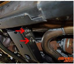
7. We then made sure that the transmission was securely and properly supported on a jack and a jack stand and then removed the two driver's side cross member bolts first, then removed the two passenger side bolts. At this point we lowered the cross member on the driver's side and slide it out towards the driver's side.
