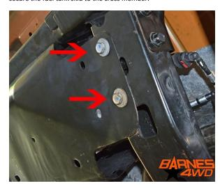
4. Using the 16mm deep well socket we removed the 3 nuts that hold the transmission mount to the cross member (one nut is not shown in picture).
