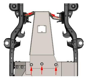
Install the oil change access panel using the provided 5/16"x1" countersunk screw.
