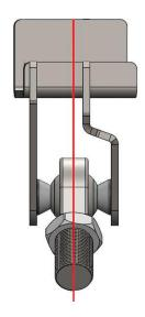
For different mounting widths. Both the Tj Track Bar Bracket Flat Tab and the Tj Track Bar Bracket Bent Tab will have to be adjusted, referencing this centerline to accommodate smaller or larger widths.
