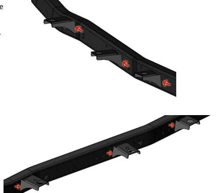
Step 3: Tack weld the top cap on the body mounts as shown in the picture below.
