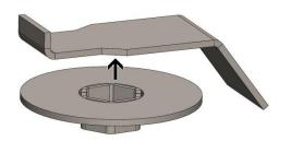
Weld around bottom of Stretch Perch on both sides.
