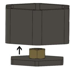
Weld the Mount Cap to the Center Halves flush. Welding on the inside of the cap.
