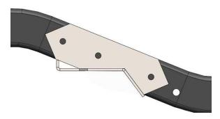
Make sure Stretch Perch edge is offset 1/4" inch with Frame Reinforcement Plate. As pictured below. DO NOT WELD IN PLACE YET.
