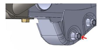
Step 2: Install the Barne4WD steering box skid onto the bumper using the provided hardware.
