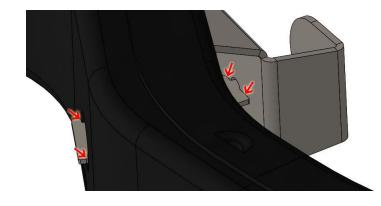
Step 5: Tack weld the bracket into place in the locations shown in the pictures below.
