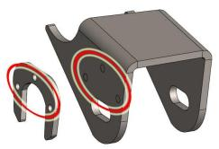
Weld into place filling the holes with weld, and welding around the outside of the cam plate.
