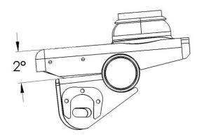
From the top of the coil spring base, to the top of the Barnes 4WD lower control arm bracket will have an angle of 2°. (See image above.) This measurement will be the same for both Barnes 4WD lower control arm brackets.
