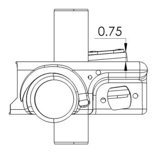
From The edge of the coil spring base, to the corner of the Barnes 4WD lower control bracket will measure ¾" of an inch. (See image above.) This measurement will be the same for both Barnes 4WD lower control arm brackets.
