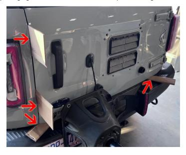
**Step 4:**Remove the 4 bolts holding the hinges to the tailgate.
