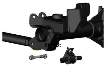
Slide the Rear Axle lower control arm bracket kid onto the bracket and install with the provided control arm bolts and factory sway bar bolts. The factory brackets typically flare out and will need to be pulled together to place the skid plates in position.
