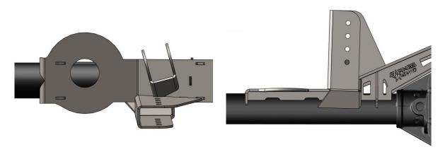
Install the track bar bracket. The track bar bracket will be placed on the backside of the truss, it will locate with a tab on the bottom of the bracket in a slot on the top of the truss. Tack weld the bracket when positioned correctly.
