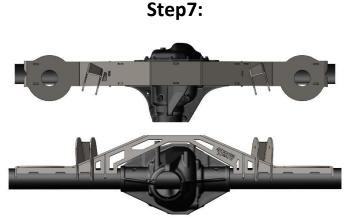
Add the upper control arm brackets to the truss. Place the upper control arm brackets on top of the truss as shown in the image below. Slide the brackets down the truss until they are in their correct position. When placed correctly they should contact the truss and the axle tubes, tack both brackets in place.
