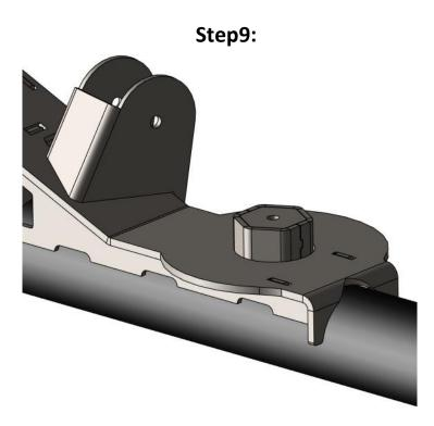
Install coil spring caps and nut assembly from step 5 in the holes on either side of the truss and tack weld in place.
