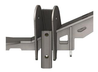
Install the sway bar bracket assemblies from step 6. Place the brackets on the axle tube inside the upper control arm brackets. The sway bar brackets should be vertical, and the upper inside corner should touch the inside of the upper control arm bracket on the side closest to the pinion. When positioned correctly tack weld the brackets to the axle tube.
