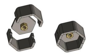
The 3/8" nuts provided in the kit need to be welded to the coil spring caps. Center one nut on one coil spring cap and weld the nut to the cap, repeat this step for the other coil spring cap. Now the assembly is ready to be welded as shown above.
