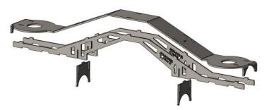
Tack weld the top, sides, and the two gussets of the truss together. The tabs on the angle section of the side plates will appear not to line up. You will need to flex the top of the truss to line the tabs up to insert in the holes. After the center 3 tabs are inserted in the truss top use a clamp to pull the outer two tabs in. Repeat this for the other side plate.
