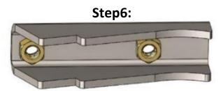
The sway bar brackets will also need nuts welded to the backside. Place one 3/8" nut over each hole on the backside of each bracket and weld in place.
