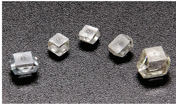
Laboratory-grown rough diamond crystals created by the HPHT process display a distinctly different shape than natural rough diamonds.
