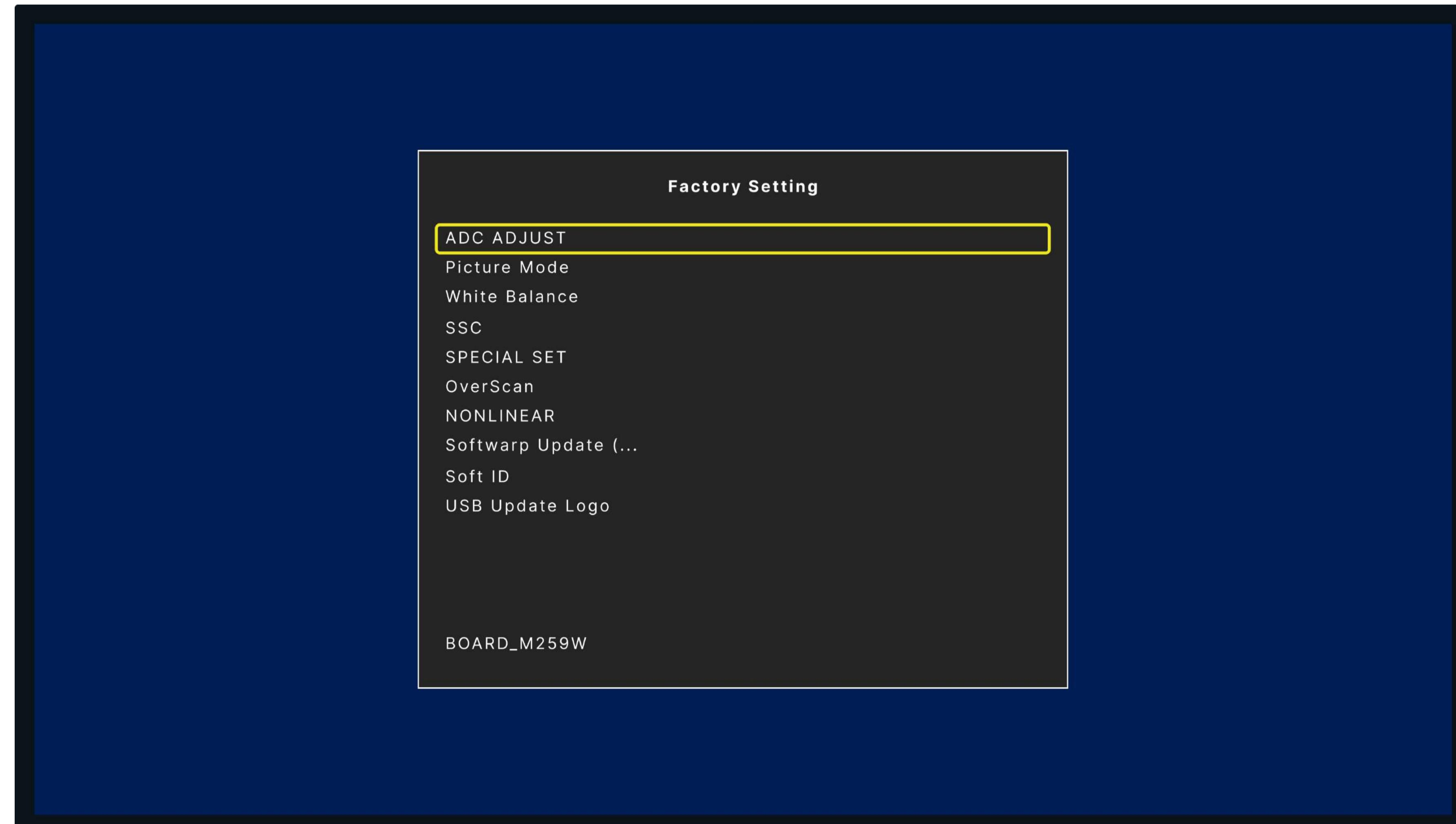
The ADC is adjusted to be automatically corrected by the front-end analog-to-digital conversion circuit under the VGA channel, and it can also be adjusted manually, but manual adjustment is not recommended. It is recommended to do AUTO ADC operation on the basis of the gray scale or color bar test screen under VGA to automatically correct the parameters of the digital-to-analog conversion circuit .
