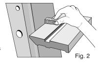
into the tubes (FIG. 2). If any excess glue remains inside the tubes it should be gently scraped out.
