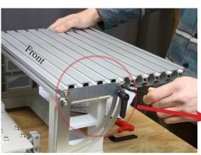
Begin by removing the Centering Scale Fence and mark the front of the table using a pencil or piece of tape so the table can be re-installed the
