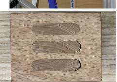
The three steps in the mortise slot allow three widths of mortise. Use the lowest step when you need a perfect fit side-to-side for through mortise and tenon. Use the second or third step if you prefer a little side-to-side adjustability. This can sometimes be helpful during glue-up. Using the third step also allows room to wedge the tenon.
