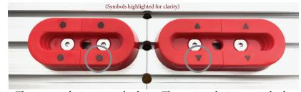
The two end pieces marked with circles make a 1" wide M&T at 3/8" thick. The two end pieces marked with triangles make a 1-1/4" wide M&T at 3/8" thick.
