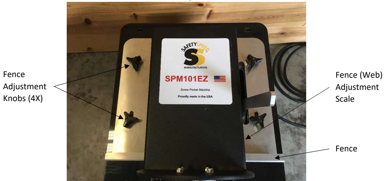
Figure 23: Fence (Web) Adjustment
