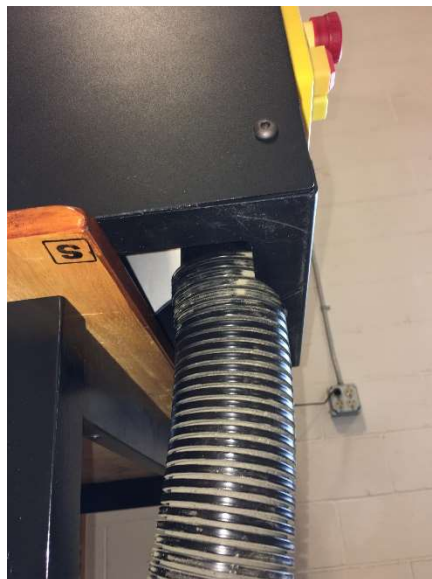
Figure 29: Dust Hose Connected (Not Supplied)
