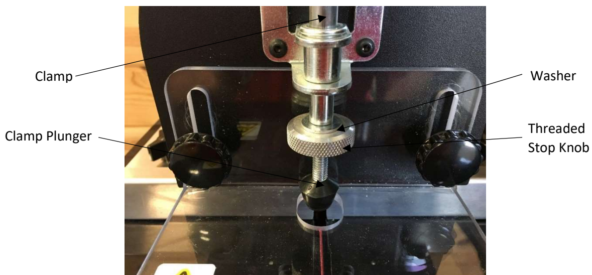
Figure 15: Adjusting the Clamp Plunger
