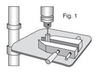
are easily drilled using a clamp and a drill press (FIG. 1). Before you start to drill be sure that your blank is at 90° to the drill press table. You may also chuck and drill the stock on your lathe.
