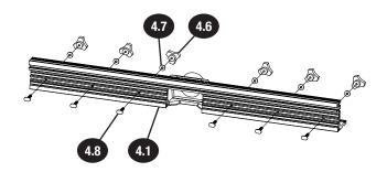
Slide the T-slot in the back of a router fence face plate (4.14) onto three of the T-bolts (4.8) you just installed.
