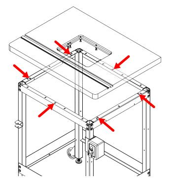
Insert a socket head cap screw (L) up through a lock washer (U) and a washer (K), then up through an elongated hole in the floor stand and into a threaded hole in the underside of the cast iron table. Repeat this process for the remaining five threaded holes in the cast iron table. Then use a 5mm hex wrench to tighten the screws.
