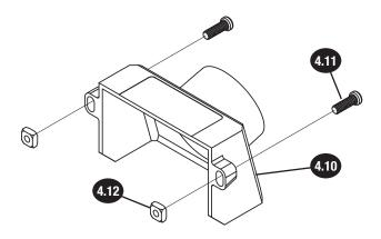
9 Slide the two ¼" - 20 square nuts (4.12) into the lower T-slot on the back of the router table fence (4.1) until the dust port is aligned with the large opening in the back of the fence. Use a Phillips screwdriver to tighten the screws to secure the dust port to the router table fence.
