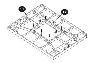
Finger tighten the hex nuts up against the bottom of the table. You will adjust the screws and fully tighten the hex nuts later, after installing the router lift.
