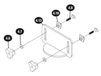
Slide the heads of the T-bolts into the top T-slot in the front of the vertical section of the router fence (4.1). The semicircular, bent portion of the router fence guard (4.15) should face away from the router table fence. The height of the router fence guard relative to the router table can be adjusted by loosening the lock knobs, moving the router fence guard up or down, and retightening the lock knobs.
