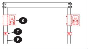
Insert a socket head cap screw (R) through a washer (K), then through the square hole in the handle mounting bracket (T). Then thread the screw into one of the single holes in the front of either front stand leg (F) (marked as holes "bb" in the hole pattern reference figure in step 7). Use a 5mm hex wrench to tighten the screw. (The handle mounting bracket (T) is adjustable and can be aligned any way the user desires to hold the router lift elevation handle.)
