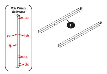
Refer to the hole pattern reference figure from step 7 and align the mounting holes in the other upper side bracket (E) with the stand leg (F) holes marked "aa" and align the mounting holes in the other lower side bracket (B) with the holes marked "cc." Mount the brackets to the stand legs using eight hex head bolts (V) and eight washers (K).
