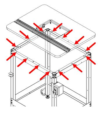
Insert a socket head cap screw (L) up through a lock washer (U) and a washer (K), then up through an elongated hole in the floor stand and into a threaded hole in the underside of the phenolic table. Repeat this process for the remaining thirteen threaded holes in the phenolic table. Then use a 5mm hex wrench to tighten the screws.
