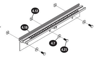
2 Slide the three square nuts (4.12) into the T slot in a rail mounting bracket (4.20). Make sure the elongated holes in the rail mounting bracket (4.20) are on the top edge. Use a 10mm wrench to tighten the hex head bolts (4.21).
