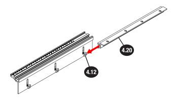
Place the rail and bracket on the side of your router table, so the four holes in the rail mounting bracket align with the four threaded holes in the underside of the router table. Use four socket head cap screws (4.23) to secure the rail mounting bracket (4.20) to the underside of your router table. Hold the 32" table rail flush with the edge of your router table, and use a 5mm hex wrench to tighten the four socket head cap screws (4.23).
