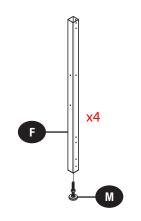
Place two stand legs (F) on a flat surface and position them so the top surface of each tube and the outward-facing surface of each tube have the holes marked as "aa," "bb," "cc," and "dd" in the hole pattern reference figure.
