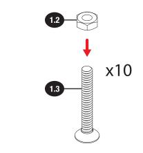
Place the router table (1.1) upside down on a flat surface and thread the flat head Phillips screws (1.2) into the threaded holes around the insert opening in the table until they extend about ¼" below the table's top surface. These screws will support and level the router lift relative to the table top. The 2 holes in the center of the short ends of the opening (indicated by the red arrows) do not receive leveling screws; they will be used later to attach the router lift to the router table.
