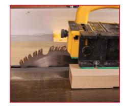
2. At the trailing end, the blade is significantly above the stock surface and just barely clears the underside of the GRR-RIPPER. In this case, shifting the GRR-RIPPER forward provides just enough clearance for a safe cut.
