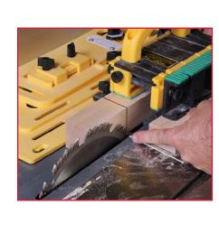
4 sides of the leg then tilt the saw blade to 45-degrees and reset the jig to the desired rise and run or degree. Notice the bigger the angle will result in a steeper taper cut. Use your best judgment on the style and design of your tapers. In the example image, the piece tapers to an octagon at the bottom, so the setting was 3 times the original taper of 3/4" per foot. Reset the fence to have the taper start in the desired place.
