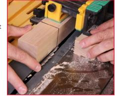
4. Make the tapers as usual, rotating the piece clockwise after each cut. NOTE: if you are using a right-tilt saw, Pay close attention to where the blade is as you will be cutting along the upper corner of the workpiece.
