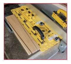
2. To cut the second side, flip the piece over so the side you just cut is against the jig. Lay out the second cut. Reset the jig to double (2X) the setting for the first cut. Here the setting is for 6°. Secure the piece the table with your hand. Keep fingers clear of blade. Make the cut. Note: You may need to adjust the rip fence to align the saw blade to the starting point of the second taper.
