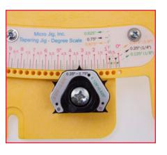
2. To set the scale, lift up on the adjustment knob and pivot it. For whole and half degrees, use the pointer marked with the red 0.
