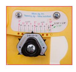
**4.** For the sixteenths, use either the pointer near the yellow or green numbers aligned with the yellow or green lines respectively. Here the jig is set to cut a taper of 1 3/16" per foot.
