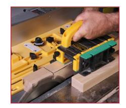
6. On most tapered legs, the two tapered sides are adjacent to each other. This means the leg will be thinner after you rotate it to get ready to make the second cut. To compensate for this, loosen the knobs on the sides of the GRR-RIPPER and push it down so it makes firm contact with the leg. Tighten the knobs to lock the GRR-RIPPER in place.
