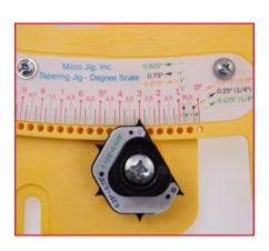
**5.** For angles that fall in between the eighths, use the pointer marked with a black X inside a circle.
