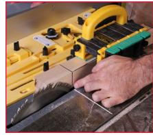
saw blade no more than 1/4" (.25") above the surface of the workpiece. Ensure that the saw blade passes through the GRR-RIPPER tunnel.
