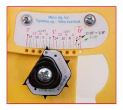
Your MICRODIAL Tapering Jig is factory calibrated and ready to go. In the unlikely event that the MICRODIAL scales are not aligned properly, follow these steps to recalibrate the jig to make the scales accurate once more.
