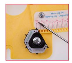
Sometimes it is easier to simply layout the taper on your workpiece and then cut to that line. To set your MICRODIAL Tapering Jig to cut to a line, lay out the taper on the face of your workpiece. Extend the layout line down the ends and/or edges of the piece so you can see exactly where you want the taper to begin and end. NOTE: Once you have the jig set, use the degree scale to determine the actual measurement and record it in your Project Log (page 28).
