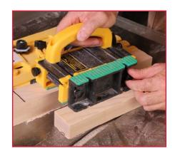
7. For longer workpieces, adding a second GRR-RIPPER gives you increased control. Tie the two GRR-RIPPERs together with a longer riser block. Just make sure both GRR-RIPPERs will clear the blade.
