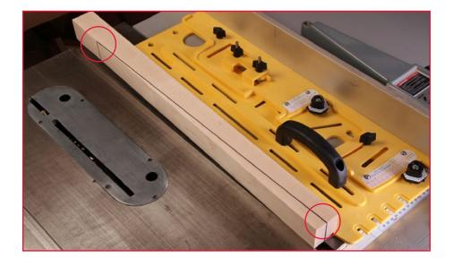
Lay out the taper on your workpiece. Hold the piece on your saw so the beginning and end points align with the edge of the miter gauge slot (which should be parallel to the blade).
