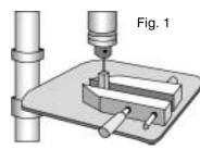
easily drilled using a clamp and a drill press (FIG. 1). Before you start to drill be sure that your blank is at 90° to the drill press table. You may also chuck and drill the stock on your lathe.
