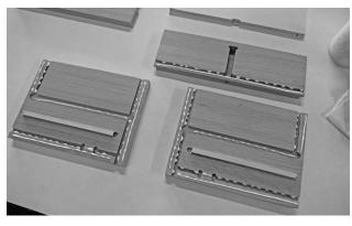
Make sure you DO NOT get any glue inside the plunger pin pocket shown here. Any glue in this area will prevent the plunger pin from working properly.
