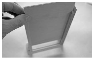
Make sure all parts are flush to the top edge then clamp drawer for proper assembly. Check drawer for square.
