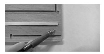
Make sure any excess glue is removed so it does not interfere with the function of the drawer.
