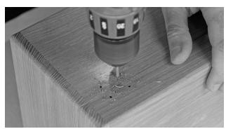
Carefully flip chest and top over so that the front of the box is facing upwards. To locate and drill for the lock, the lock will need to be positioned on the centerline of the chest. It might be helpful to start with the lower half of the lock and screw it down first. Then position the top half of the lock and drill for the screws. Screwing the bottom half down helps keep things in position, reducing the chance of error.
