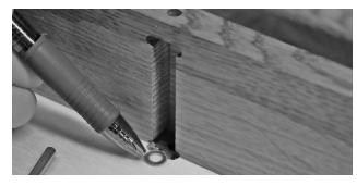
Using a pair of needle nose pliers, push the end of the pin through the bottom washer and release it through the top hole. This can be a bit awkward and challenging so several attempts might be necessary. Scan the QR code above to see a video of this process.
