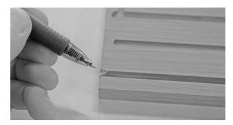
The sides, front rail and back have been marked with matching indicators to ensure the proper orientation of parts. They could be lettered pairs or number pairs.
