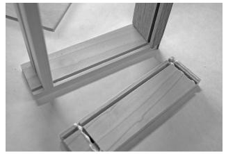
Slide the drawer bottom into place and install the remaining drawer side.
