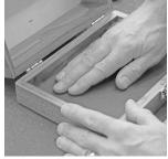
The surround strips are installed one at a time and will overlap in the corners.
