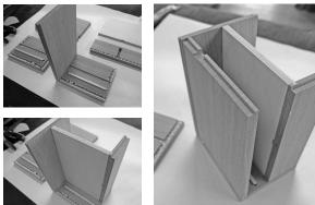
Install the remaining side and make sure all parts are flush to the top edge. Clamp parts and check for square.
