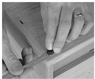
Locate and mark the center of the drawer front. Drill a 3/16" hole for the knob.
