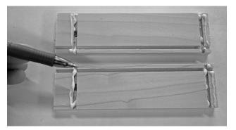
Install the drawer front and drawer back. Make sure the drawer bottom grooves are in alignment.
