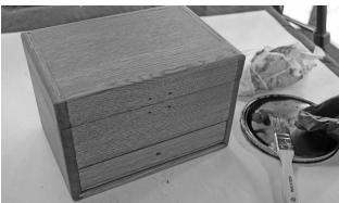
Apply a lacquer finish to the chest. Lightly sand the first coat, or seal coat, once dry with 320 grit sand paper.
