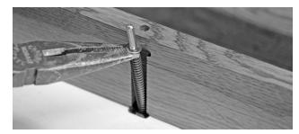
Install the chest hardware. DO NOT over-tighten the screws or you will damage the hardware. Drive the screw in until it makes contact with the hardware and stop.
