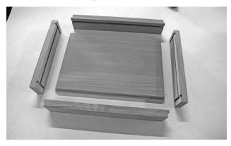
Apply glue to both the shoulders and grooves of the top parts.
