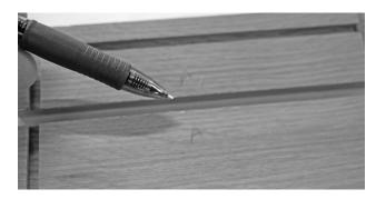
Glue the maple drawer slides into the sides, making sure that they are positioned all the way forward in the groove. Any gap should be to the back of the chest.
