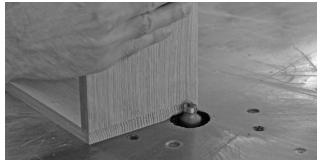
Sand and fit the drawer to the chest. Make sure it operates freely and has the minimal amount of gap. The minimum gap is 1/32". We recommend between 1/32-1/16".
