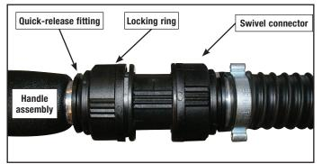
Figure 2. With locking ring unscrewed (as pictured) depress quick release ring then pull quick-release fitting toward hose.
