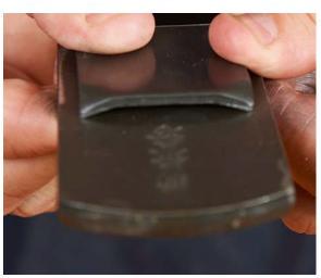
Because of the shrinkage of the plane body, initially it is unlikely the plane iron will protrude through the sole.
