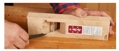
Remove and carefully pare, scrape or rasp the area of the Dai marked with the pencil lead until it is removed. Replace the iron, and check if it is now within 1/16" of the opening. If not, repeat the above procedure. Normally two or three times will suffice. Check the sole from time to time to ensure it has remained flat.
