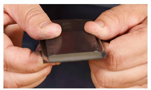
breaker over and sharpen at an angle of 20° on a coarse water stone until the edge is sharp, then polish the bevel and hollow side on a finish stone. Finally, hold the chip breaker at an 85° angle to the finish stone and make a dozen or so strokes. This will add a secondary or "micro bevel" on the chip breaker. The ideal chip breaker breaks the shaving without offering any further resistance.
