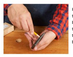
Replace the iron and push it by hand into the Dai as far as possible. Inspect the opening at the sole . If the iron is within 1/16" of the opening, it should be possible to tap the top of the iron with a mallet or small hammer until the edge protrudes through the sole. If the edge is greater than 1/16" from the opening, remove the iron and rub a soft lead pencil on the sides and back of the iron. Now push the iron by hand as far as possible into the body.
