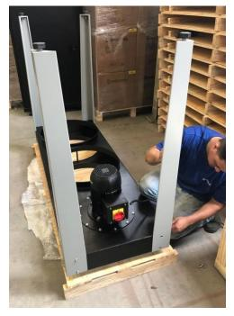
3. With help of someone turn the dust collector to the correct position, as shown below images:
