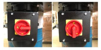
2. Turn on the machine and quickly turn it off, check the impeller looking into the 5 port splitter and confirm if the motor is spinning in the correct direction, as the sign bellow indicates:
