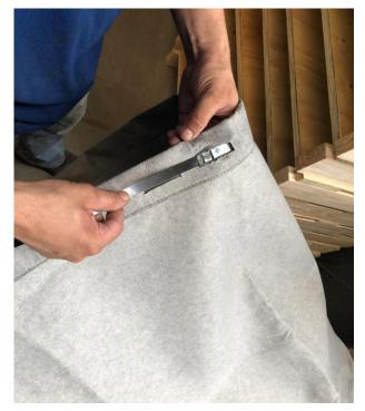
8. Slide the filter bag loop over the hanger hook (repeat this process twice):
