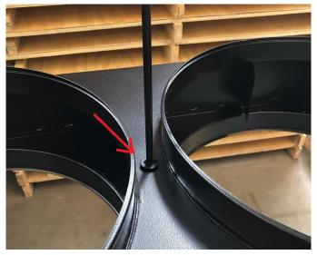
6. To assemble the 5 port splitter, apply silicone to the area around the main orifice then use the 12 piece hardware kit to fasten the port splitter to the main orifice (**silicone not included**):
