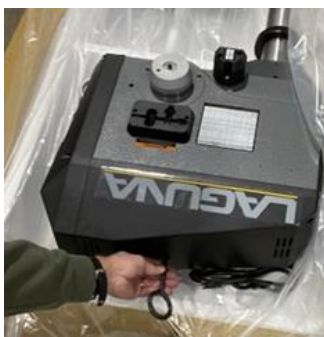
Figure 15: Installing Lifting Eye
