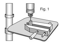
are easily drilled using a clamp and a drill press (FIG. 1). Before you start to drill be sure that your blank is at 90° to the drill press table. You may also chuck and drill the stock on your lathe.
