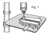
are easily drilled using a clamp and a drill press (FIG. 1). Before you start to drill be sure that your blank is at 90° to the drill press table. You may also chuck and drill the stock on your lathe.
