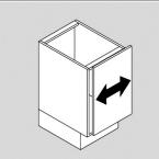
Rotate the front screw to increase or decrease the door overlay (+/- 2 mm).
