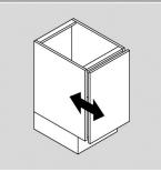
Rotate the rear spiral tech cam screw to adjust the door position (+ 3/- 2 mm).
