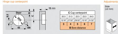
Cup centerpoint is the MINIPRESS or MINIDRILL fence depth position.
