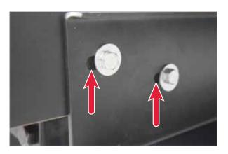
Using a 10mm wrench on the head of each bolt and an 10mm wrench on each nut, tighten the nuts on the bolts to secure the dust collection guard mounting bracket to the extension table.
