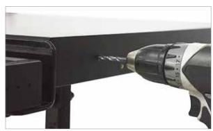
Place the flat edge of the dust collection guard mounting bracket (B) in the same position as in step 2, with the mounting holes aligned with your drilled through-holes.
