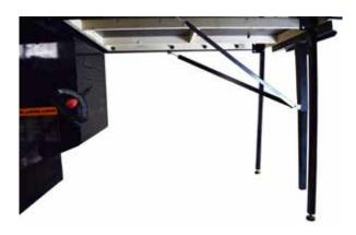
Check to make sure the extension leg is still vertical and make any necessary adjustments.
