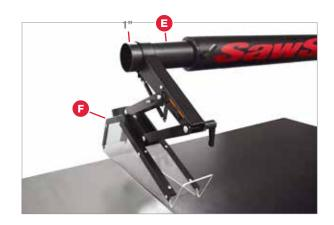
Slide a M6 x 1.0 x 40 button head socket screw (T) through the two holes in the clamping portion of the floating blade guard (F), with the threaded portion of the bolt facing towards the front of the floating blade guard.
