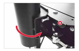
Grasp the end of the 3/8"-16 dust tube lock knob and pivot it towards the dust tube assembly until the end of the threaded portion of the lock knob lines up with the depression in the flat plate portion of the outer dust tube (D) and push it until it is over center past the depression.
