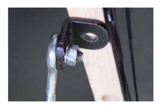
Insert a M5 x 2.1 x 32 button head Phillips screw (S) through a M5 x 12 x 1 washer (R) and then through the exposed hole in the leg support mounting bracket (O). Secure the bracket to the underside of the extension table support frame using a Phillips screwdriver or drill.
