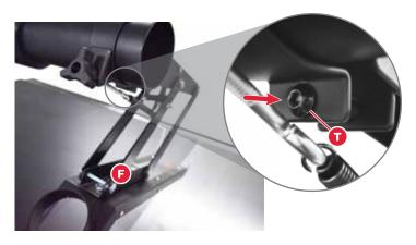
It may be useful to loosen the spring tension knob on the rear side of the clamping portion of the floating blade guard so the spring can be pushed out of the way.
