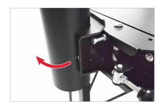
Loosen the 5/16"-18 nut using a 1/2" wrench and thread the 5/16"-18 x 1-1/2" hex head bolt in or out relative to the dust collection guard mounting bracket. Once the bolt is in the correct position, use a 1/2" wrench to re-tighten the nut in order to secure the bolt.
