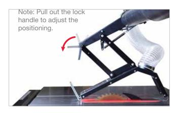
Move the floating blade guard up or down to the desired position and then tighten the lock handle by rotating it in a clockwise direction.
