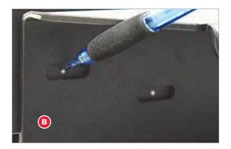
Use a 1/4" drill bit to drill four through-holes in the extension table at the locations marked in step 3.
