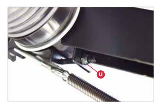
Lock the floating blade guard in its upper, retracted position. To do this, loosen the floating guard lock handle and lift the clear hood portion up towards the inner dust tube. When the floating blade guard (F) is in its upper position, re-tighten the floating guard lock handle.
