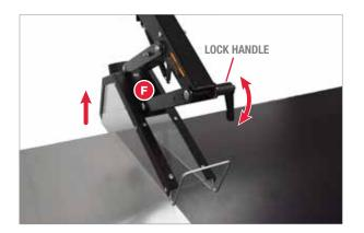
Loosen the inner dust tube lock knob and extend or retract the inner dust tube (E) to center the floating blade guard (F) over the blade. Then re-tighten the inner dust tube lock knob to secure the inner dust tube and floating blade guard.
