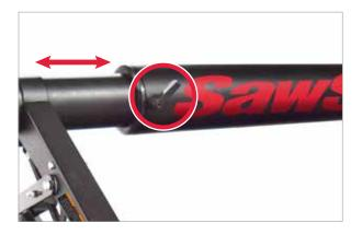
Tighten the inner dust tube lock knob by turning the handle clockwise. Do not over-tighten the inner dust tube lock knob.
