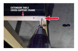
Pivot the leg support bracket and attached components up again and align the leg support mounting bracket hole with your drilled pilot hole.
