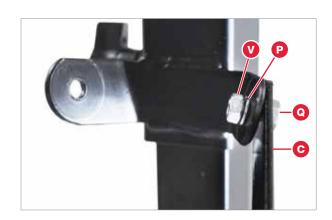
Repeat steps 1-2 to attach the other leg support bracket (C) to the exterior side of the rear tab, making sure the bent sections of the leg support bracket and the leg support mounting bracket face out toward the rear of the saw. Only fingertighten the nut at this time.
