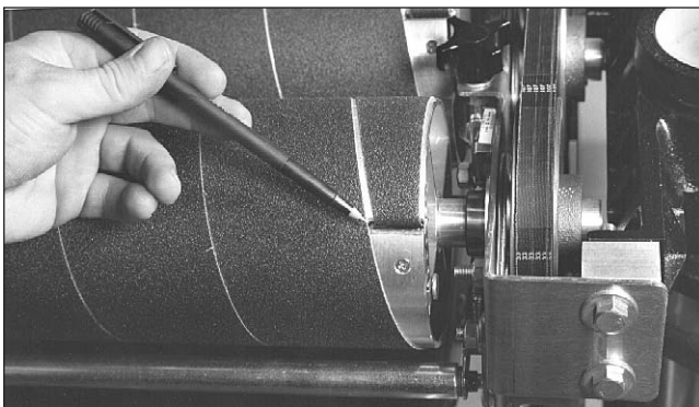
Fig. 12-h. Allow room inside slot for strip to move.
