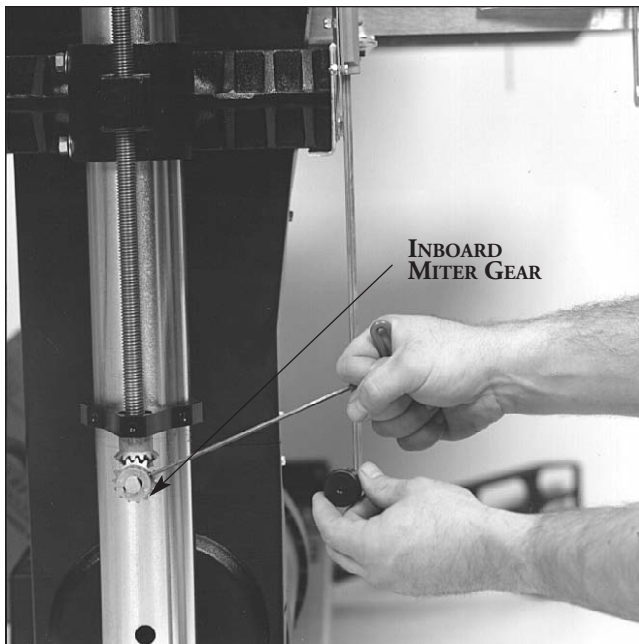
Fig. 8. Adjusting primary drum alignment.
