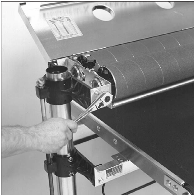
Fig. 31. Drum support casting bolts (outboard side).
