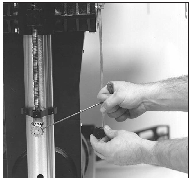
Fig. 7. Checking drum alignment (inboard side).
