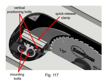
To align the spreader or riving knife so it is within the kerf of the blade, place a straight edge along the left side of the blade, making sure the straight edge runs between the teeth (see Fig. 118). Slide the clamp left or right until the left side of the spreader is flush and flat against the straight edge. If necessary, pivot the left anti-
