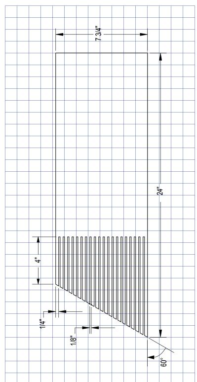
This diagram illustrates a typical featherboard. Featherboards should be constructed from good quality wood that is free of knots. Use featherboards to help keep the material being cut in contact with the table and to help prevent kickback. Do not use featherboards when cutting with the miter gauge.
