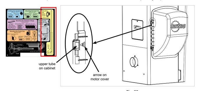
Slip the straight end of the motor cover rod up through the bottom tube then through the row of half-cylinders along the edge of the motor cover and finally through the upper tube (see Fig. 23). Rotate the motor cover rod so that the bent end of the rod fits into the hook on the motor cover just below the bottom metal tube (see Fig. 24).
