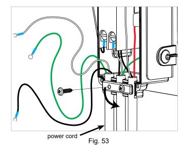
Now install the new power cord in the contactor box. Connect the ground wire (the green wire) to the ground, the white wire to the right, top terminal connection on the contactor, and the black wire to the left, top terminal connection on the contactor (see Fig. 54). A wiring diagram is shown in Fig. 55 on page 41.
