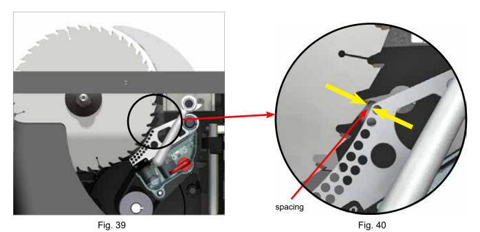
The spacing between the brake cartridge and the blade is adjusted by the yellow brake positioning bolt mounted in the top of the arbor block (see Fig. 41). To access the brake positioning bolt, set the tilt angle to  $0^{\circ}$  and adjust the blade elevation to approximately  $1\frac{1}{2}$  inches above the table top. The bolt will be accessible through the opening in the table top.
