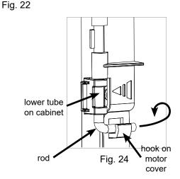
To open the motor cover press on the ribbed section on the front of the motor cover until it unlatches and swing the cover away from the cabinet. Reverse the process to close the cover (see Fig. 25).
