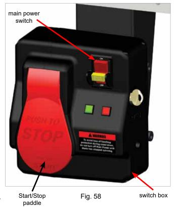
It is not necessary to turn off the main power switch after pushing in the Start/Stop paddle to turn off the motor. If you plan to make several cuts with the saw, you can leave the main power switch in the *ON* position between cuts to eliminate the delay due to the initialization routine. Once you have finished using the saw, turn the main power switch to *OFF* to reduce the likelihood of inadvertent start-up.
