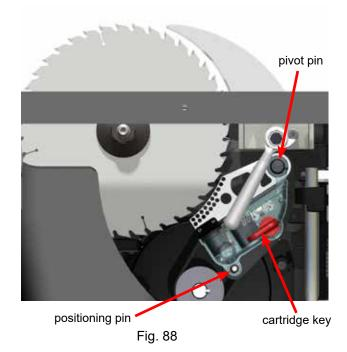
To remove the cartridge, first remove the cartridge key by turning it 90° clockwise and then pulling it away from the cartridge (see Fig. 89). Set the cartridge key aside for use with the new cartridge.
