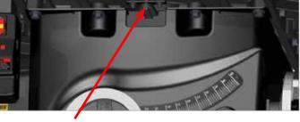
The pivot pin is pressed into this boss
