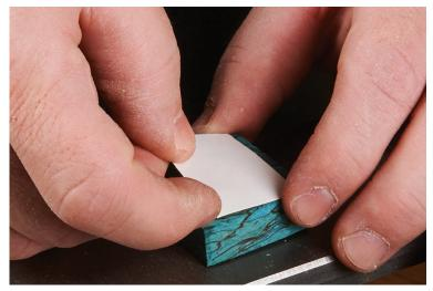
Center the blank on the live center, and advance against the face of the scrap block. The pressure of the live center will enhance the bond of the tape during the rough turning process.
