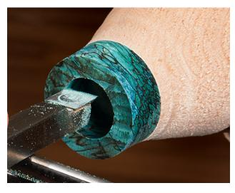
When the ring core fits the opening, true the face of the blank to the same width of the ring core, ensuring a good fit.
