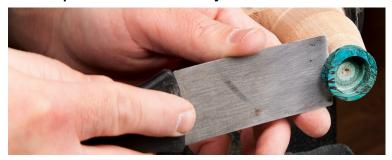
Apply a light coat of either thick CA glue or 5-minute epoxy (recommended) to both the ring core and blank. Immediately remove any excess glue.
