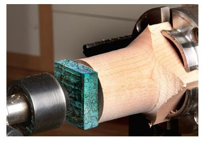
Rough turn the blank to round. Remove the live center.
