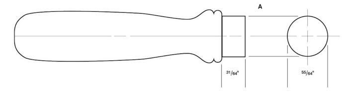
With the lathe spinning, begin sanding with 120-grit paper progressing through the finer grits, finishing at 320-grit. Once finished with sanding, apply a finish of your choice.
