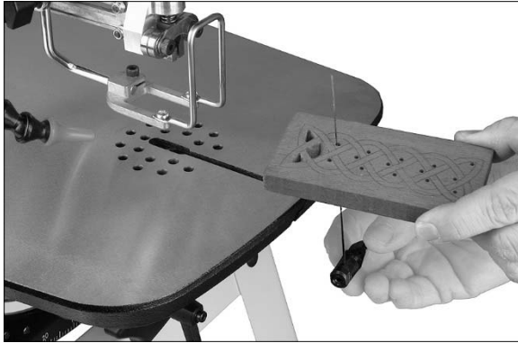
Figure 16: installing blade with workpiece
