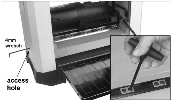
Figure 8-4: knife insert rotation/replacement
