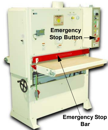
Figure 18: 37" x 60" Belt Sander Emergency Stops
