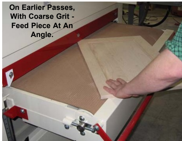
Figure 46: Angle Feed
