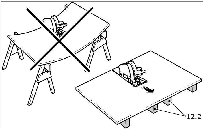
Never position large or long workpieces so that they bend in the middle or at the cutting face. This can lead to the saw blade jamming and recoiling. Instead, support the workpiece with several wooden battens (12.2), particularly in the vicinity of the cutting face.
