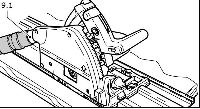
A Festool dust extractor with an extractor hose diameter of 36 mm or 27 mm (36 mm recommended due to the reduced risk of clogging) can be connected to the rotating extractor connector (9.1)
