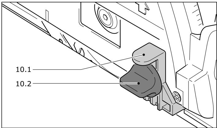
The splinterguard (accessories) significantly improves the quality of the cutting edge of the sawn workpiece on the upper side for 0° cuts.
