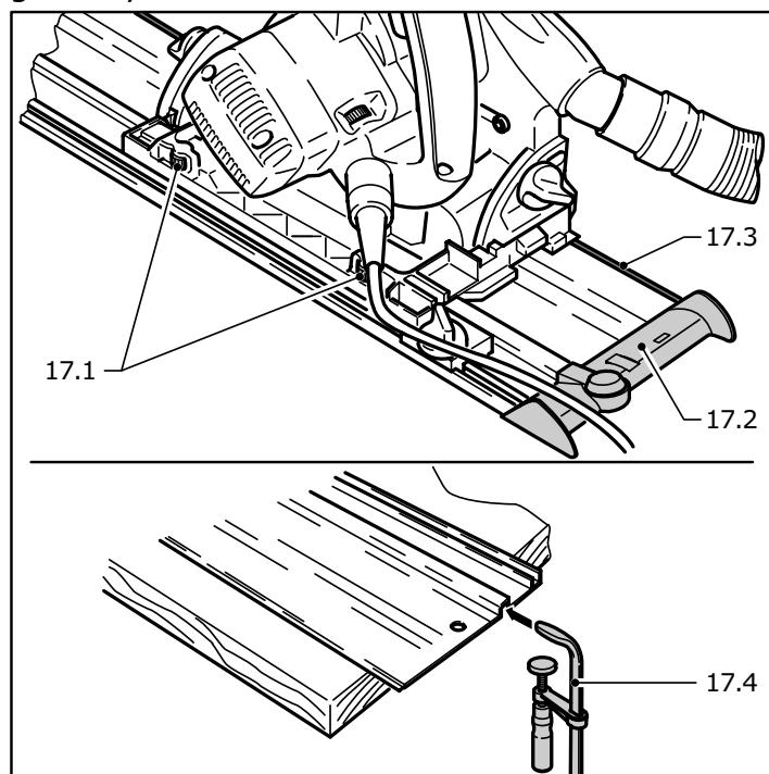
The option of securing using G-clamps (17.4) ensures a firm hold and safe working. The optional cord guide (17.2) prevents the power cord and vacuum hose from catching on the end of the guide rail.
