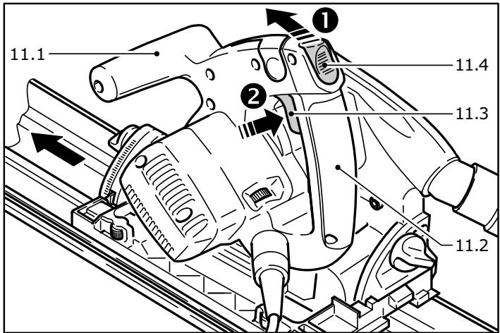
**!WARNING** Keep the machine steady during switching and during use by holding the handle (11.2) and the additional handle (11.1) with both hands.
