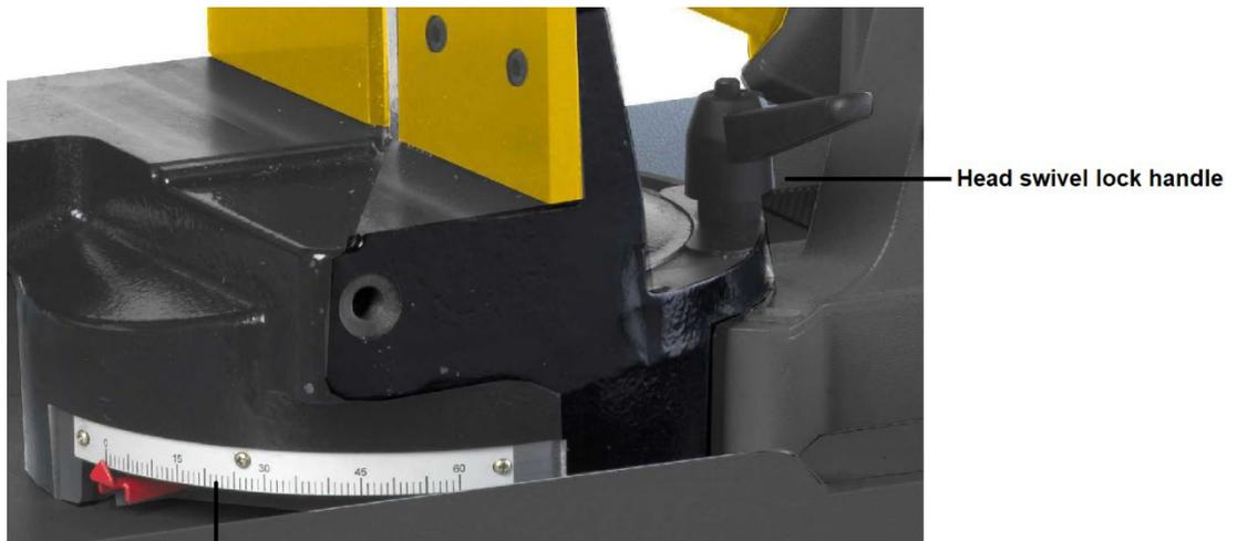
Miter scale. Preset stops at 0-45-60 degree angles.
