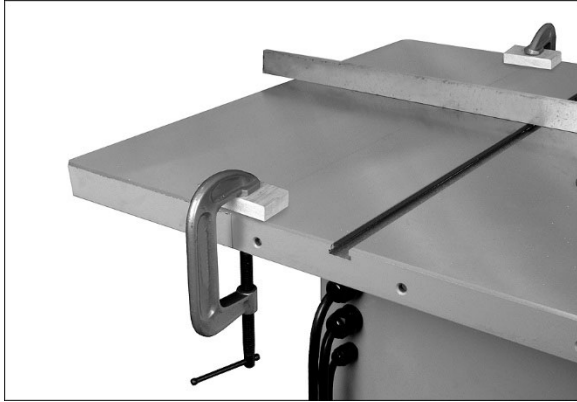
Figure 6-5: leveling extension wings, method 2
