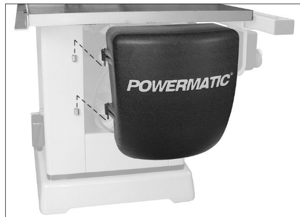
Figure 6-7: installing motor cover
