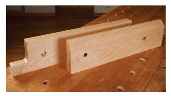
The 8" Acme screws are held to the rear jaw with two nuts and two washers on the back side and two nuts mortised into the inside face of the rear jaw. This mortise can just be a counterbore with a larger forstner bit, or you can scribe the hex shape of the nut and make a perfect fit. The hex shape mortise will make it easier to tighten the rear nut and secure the screws. Either way, be sure to mortise deep enough that the nut is completely below the surface.
