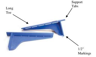
OUR MOUNTING BRACKETS ARE DESIGNED TO EASE THE PROCESS OF ALIGNING A FULL-EXTENSION DRAWER SLIDE TO THE DRAWER BOX ONCE THE SLIDE HAS BEEN MOUNTED INTO THE CABINET. BRACKETS ARE DESIGNED TO WORK WITH BOTH FACE FRAME AND FRAMELESS CABINETS.
