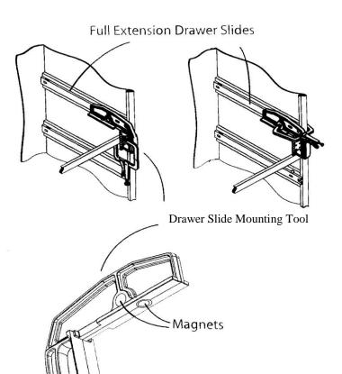
The magnet on the bottom of the mounting tool is used to locate bottom mount drawer slide as shown on the right.
