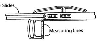
Full extension drawer slides are designed to support a lot of weight and extend all of the way out of the cabinet. The Drawer Slide Mounting Tool is ideal for accurately positioning full extension drawer slides.
