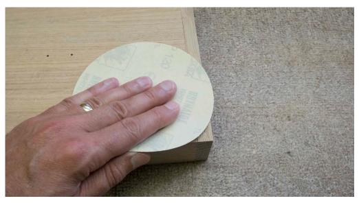
7) Sand the exterior of the box as desired. USE CAUTION when sanding the top veneer, as it is very thin and can be damaged easily!
