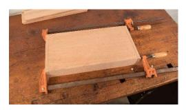
6) Next, assemble the tray as shown. The tray bottom is 1/8" birch plywood and is installed in the 1/8" groove cut in the tray parts. Please note the tray bottom will not be flush with the tray frame parts. The plywood bottom is recessed into the tray as shown in the pictures below.
