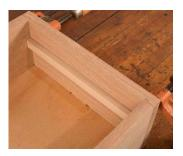
5) Lay top parts out, glue and clamp in the same way that the bottom section was completed in Step 3. Remove excess glue and check top for square. Make sure top is flush with frame parts and not installed upside down.
