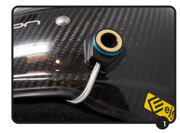
Plug the 4mm boom into the hole in the helmet side Hydro. You should feel it pop past the O-ring and shoulder against a wall. Once plugged in, bend the boom to tuck it under the helmet shell and route it behind the cheek pad, ensuring the line isn't kinked for proper fluid flow.
