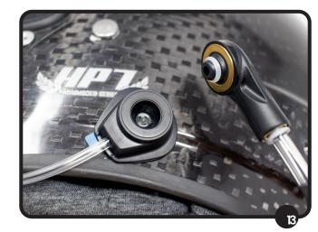
Place the helmet in the seat location and assure that the line allows for free movement. Move the helmet to the left, right, up and down. If there is excess line, remove the line from the Legris by simply depressing the gray collar and trim to fit.
