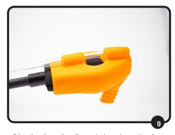
Trim the 4mm line if needed, and run the 4mm Aqua Com Line into the back of the Aqua Com. You will feel the hose seat against a shoulder in the second hole. Do not push the hose in too far as it will restrict flow.
