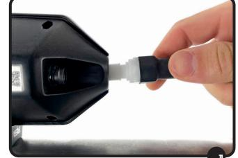
Take the male end of the CPC Connector and plug it into the output side of the Pod. It will be the side with the "C" of "FluidLogic®" on it.
