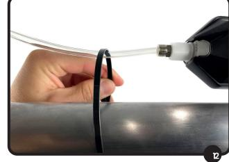
Secure the Water Line coming from the Pod towards the helmet. In this instance, using zip ties, be sure not to over tighten them as over-tightening may inhibit fluid flow.
