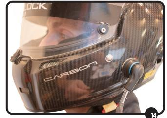
Place the helmet onto the user and test fit the HYDRO. Power and prime the system and test to make sure fluid is flowing properly. Adjust the HYDROto the user's liking.
